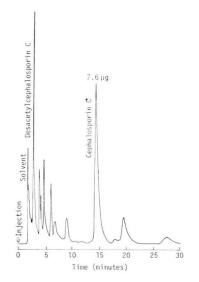
Fig. 2C. Fermentation broth on ultra high efficiency column with ion-pairing.
