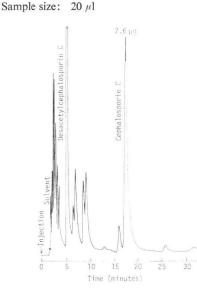
Fig. 3. Ion-pair separation of cephalosporin starting materials.
