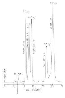
Column: 15 cm×4.6 mm i.d., C8/Lichrosorb 5 μm Mobile phase: 35% methanol - 65% 0.01 M sodium dihydrogen phosphate Pressure: 105 kg/cm<sup>2</sup> Flow: 1.0 ml/minute Detector: UV (225 nm) Sensitivity: 0.1 AUFS Sample solvent: Mobile phase Sample size: 20 μl
